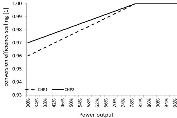
Fig. 7. Assumed conversion efficiency scaling factor for the two CHP-units
