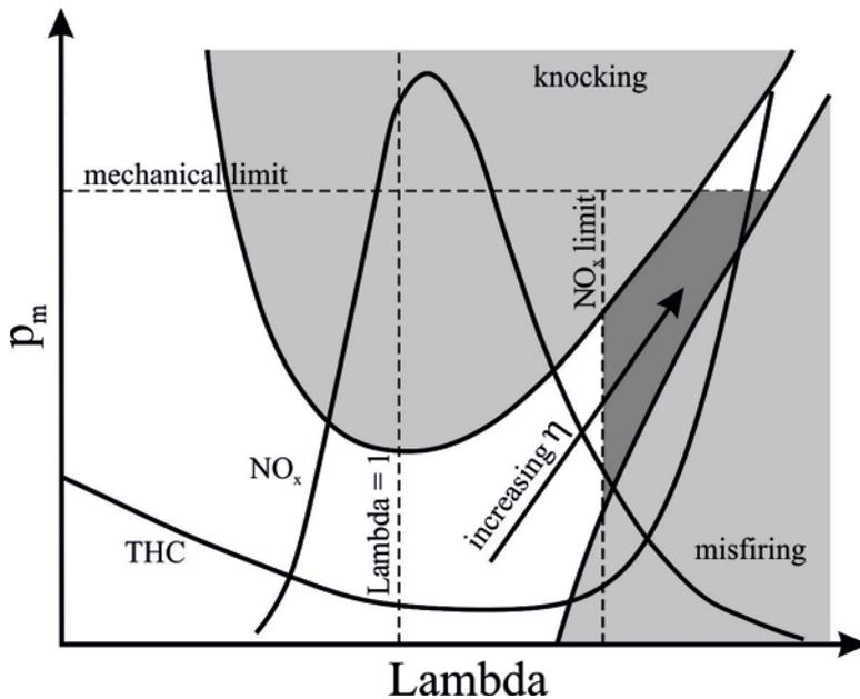
Figure 4: Operating range of gas engines [16]
