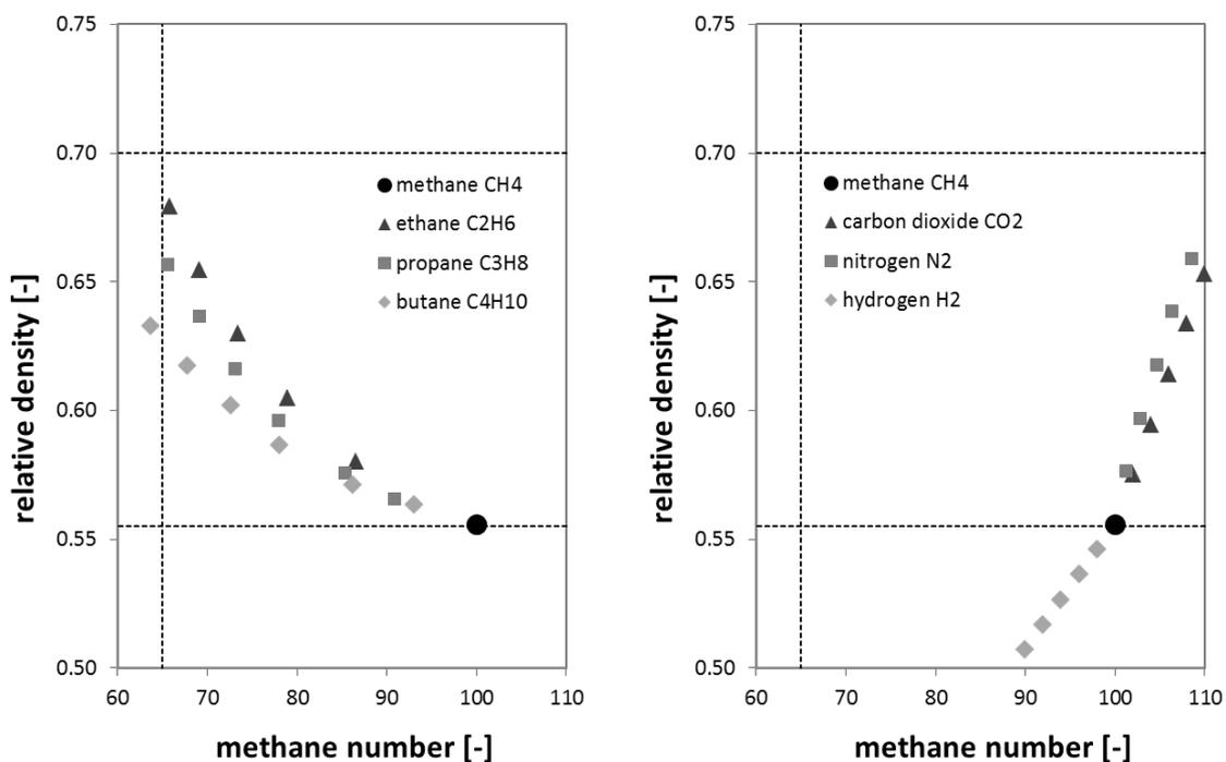
Figure 2: Mixing of selected gas components with methane and limits according to EN 16726
