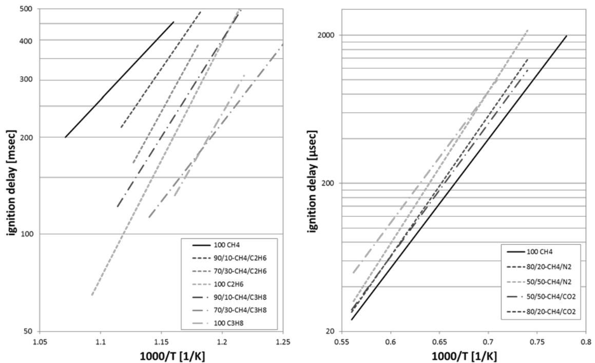
Figure 8: Ignition delay of CH<sub>4</sub> and C<sub>2</sub>H<sub>6</sub>/C<sub>3</sub>H<sub>8</sub> blends (left) & ignition delay of CH<sub>4</sub> and N<sub>2</sub>/CO<sub>2</sub> blends (right)
