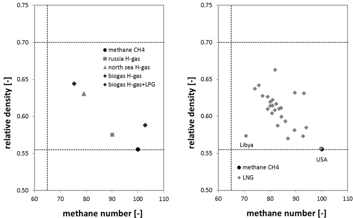
Figure 3: Different real pipeline gases and LNG compositions and limits according to EN 16726
