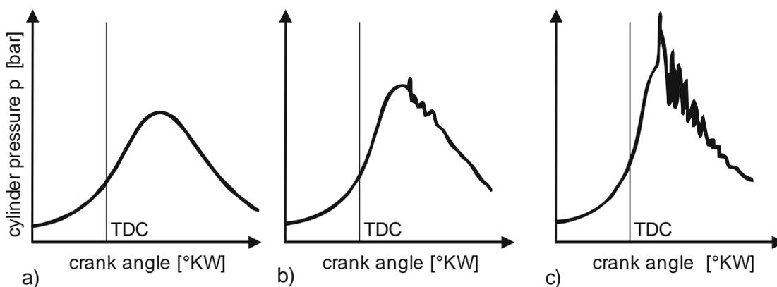
Figure 5: Comparing regular and knocking combustion [15][16]
