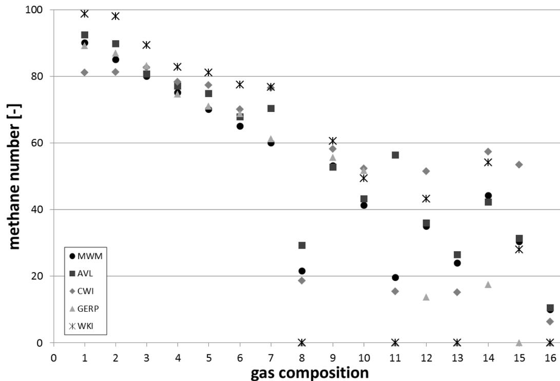
Figure 6: Methane number results of different calculation methods
