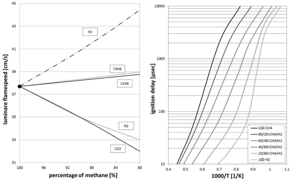
Figure 7: Laminar flame speeds of different gas compositions (left) & ignition delay of CH<sub>4</sub> and H<sub>2</sub> blends (right)
