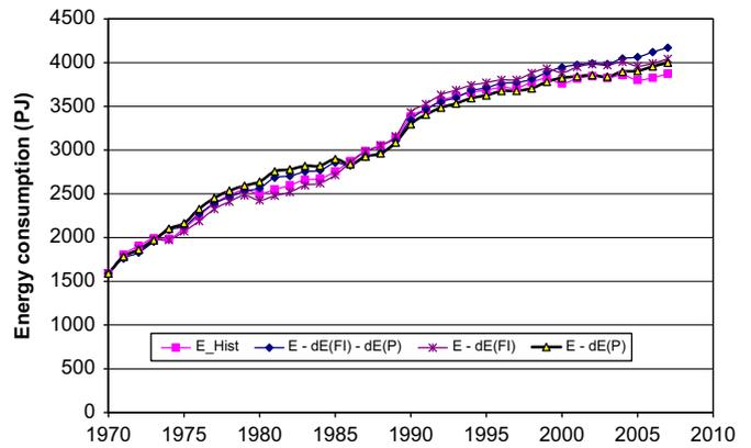
Fig. 8. Historic development of total energy consumption in comparison to the impact of fuel intensity and the fuel price for EU-6, base 1970.
