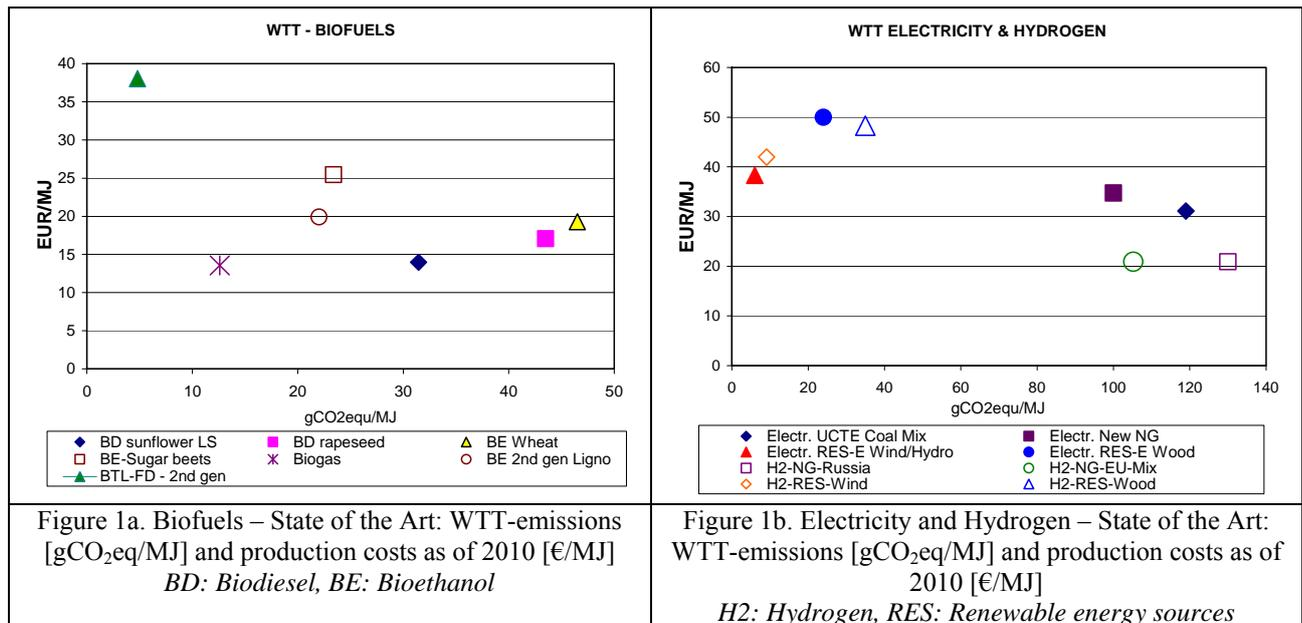
With respect to a State of the Art assessment of AAMT, the modification of the existing internal combustion engine to run on alternative fuels, able to be blended with fossil diesel and gasoline or natural gas performs differently in terms of emission reductions stating better for biodiesel and biomass-to-liquids than for gasoline or flex-fuel vehicles running on ethanol mixtures.
