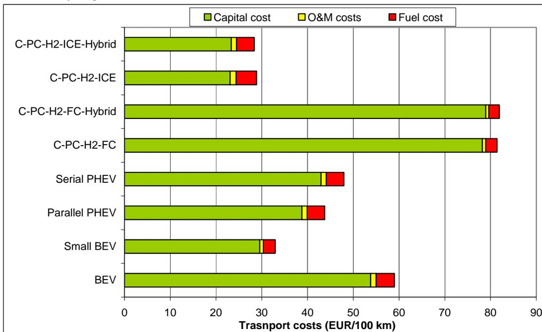
Figure 3. Hydrogen and Electric vehicles – State of the Art of economic assessment of driving costs 2010 (Size of vehicle: 80 kW except small BEV: 47 kW)
