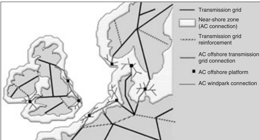
Figure 4: Common trans-national strategy for an offshore extension of the transmission grid in Northern Europe. Source: [19]
