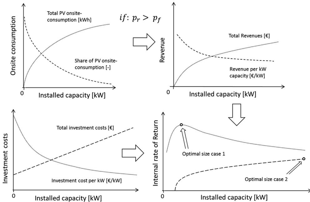
**Fig. 1.** Development of onsite consumption, revenues, investment costs and internal rate of return over PV system size for tariff structures where the value of onsite consumption is higher than the value of electricity fed into the grid.
