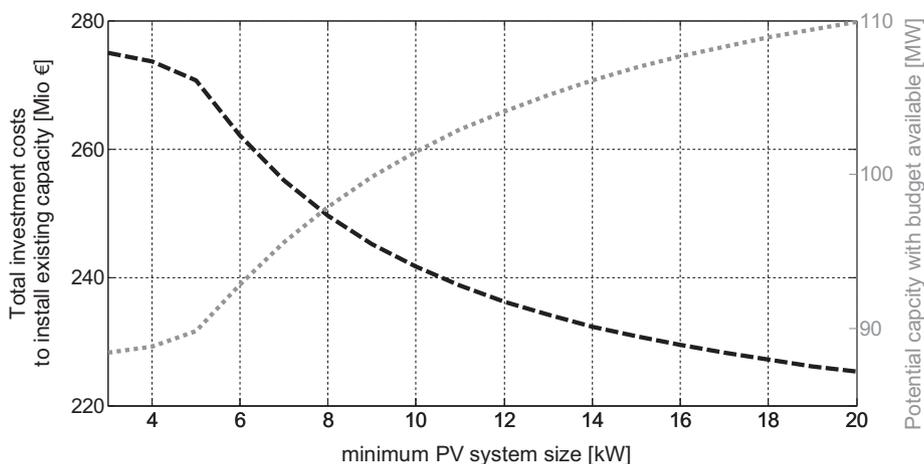
Fig. 7. Minimum PV system size and cost efficiency.
