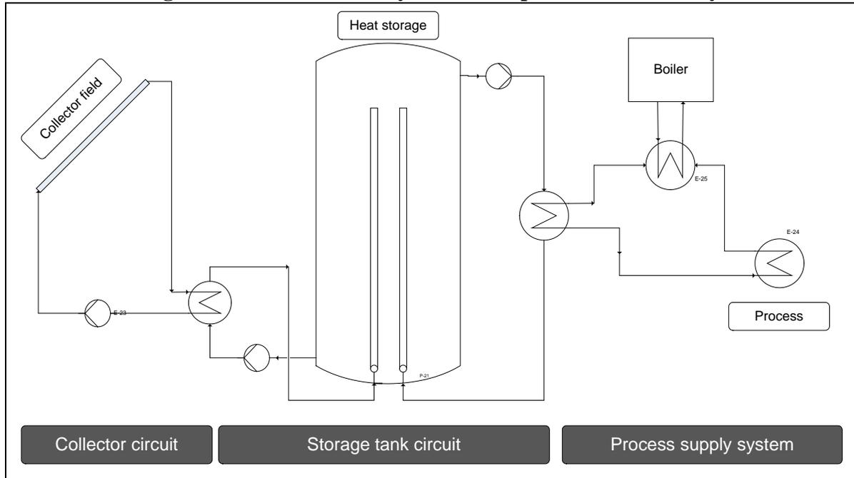
The modeled system reflects a solar thermal installation that feeds into the heat supply system of an industrial plant with one or more processes implemented at the demand side. In order to draw conclusions regarding the influence of the process load profile on the economic efficiency of the solar thermal installation for this analysis only one process is assumed at the demand side.
