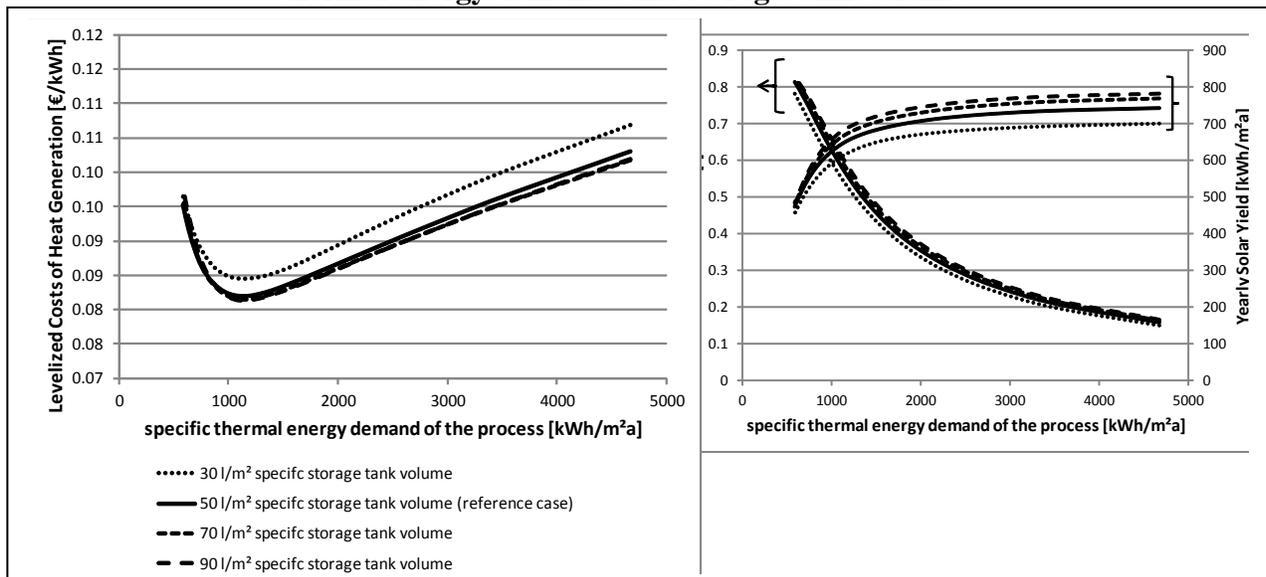
Different specific storage tank volumes are further analyzed in combination with the influence of the process load profile (Figure 5 left side). We found specific storage tank volumes between 50 and 100 l/m<sup>2</sup> to be cost optimal depending on the load profile of the process. As expected, the effect of the increase of the specific storage tank volume is higher for plants
