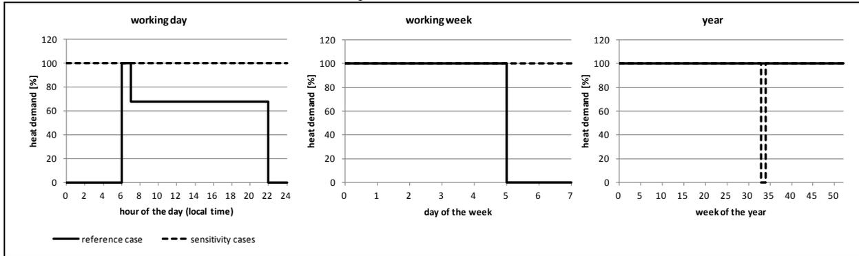
For the comparison of the performance of the solar thermal system for different load profiles and process as well as return flow temperatures the annual thermal energy demand of the process is assumed to be the same for the reference and all sensitivity scenarios. This allows drawing conclusions on the cost-optimal system size per process heat demand for different load profile and temperature scenarios.
