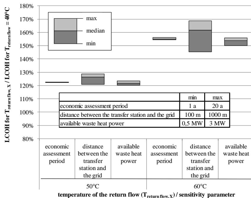
Figure 3: Relative change of the LCOH due to changes in the input parameters
