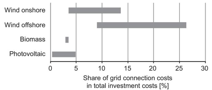
Fig. 2.1. Bandwidth of the share of grid connection costs in total investment costs. Source: Swider et al. (2008).
