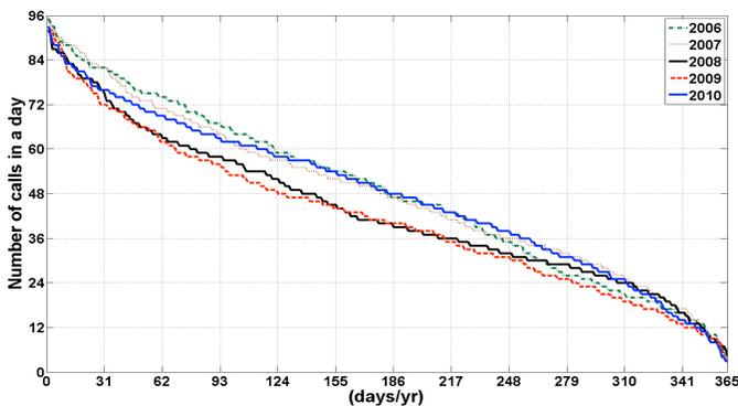
Fig. 1. Calls in the Austrian secondary (positive) control energy market for the years 2006 to 2010 [12]
