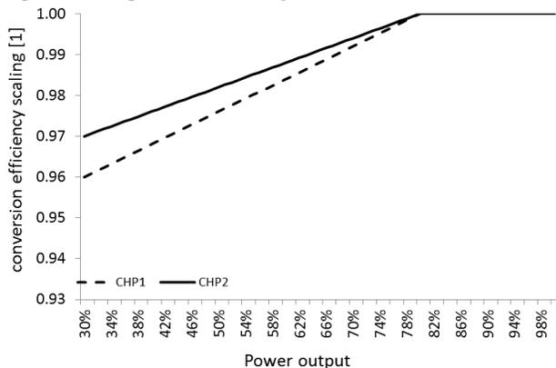
Fig. 4. Assumed conversion efficiency scaling factor for the two CHP-units
