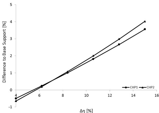
Fig. 10. Part-load efficiency variation  $\Delta\eta$  at minimal load and median market prices
