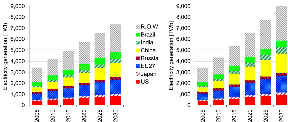
Figure 6 Comparison of the future RES-E deployment up to 2030 in absolute terms by country / region for both IEA scenarios – reference case (left) and alternative policy scenario (right)
