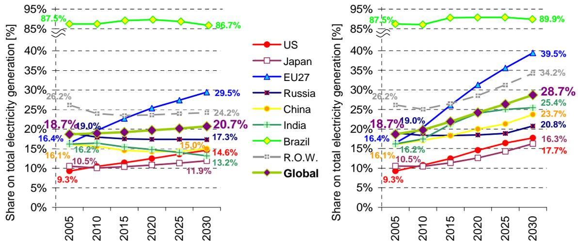
Figure 7 Comparison of the future RES-E deployment up to 2030 in relative terms (expressed as share on total electricity generation) by country / region for both IEA scenarios – reference case (left) and alternative policy scenario (right)
